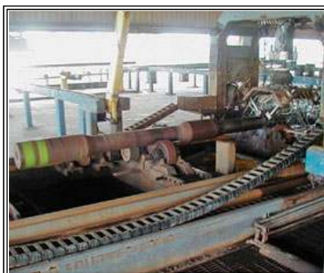
Fig. 1. Ultrasonic thickness inspection unit for advanced data acquisition on critical service drillstem components.
